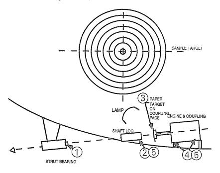
After satisfactory engine alignment as above, install shaft and its coupling, keeping shaft log propped in same position as during the optical alignment. Last, adjust engine coupling about pitch and yaw axes to acquire parallelism between two halves of coupling. Most engine specs say to within .005" difference, side-to-side and top-to-bottom. This is accomplished with tedious trials using a feeler gauge. Bolt coupling and wire securely.
