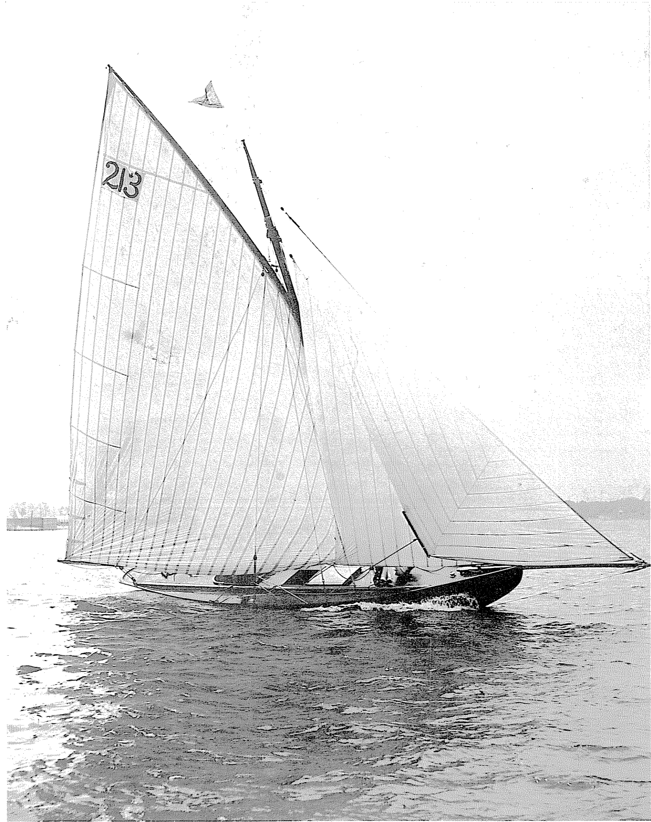
NOX, Designed by Fife of Scotland, built by Miller brothers and Meerdick in Rochester and launched in 1892, this cutter had LOA of 36 ft., beam of 8 ft. and draft of 5 ft., 6 in. During first three years she entered 16 LYRA races, winning 14 firsts. Won Madge Cup in 1892. The NOX cigar was named after this famous yacht.
